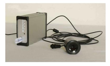
Ultrasonic playback of social and echo navigation calls can be then used for training, and the replay device potentially used for other playback purposes. ...
